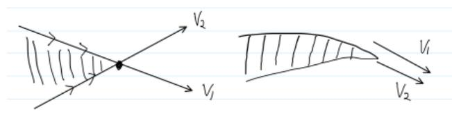
Figure: Trailing edge with finite angle and cusped trailing edge
