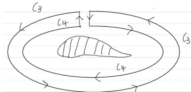
Figure: Circulation round a closed circuit that does not enclose the wing.
