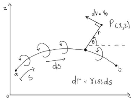
Figure: Edge view of vortex sheet
