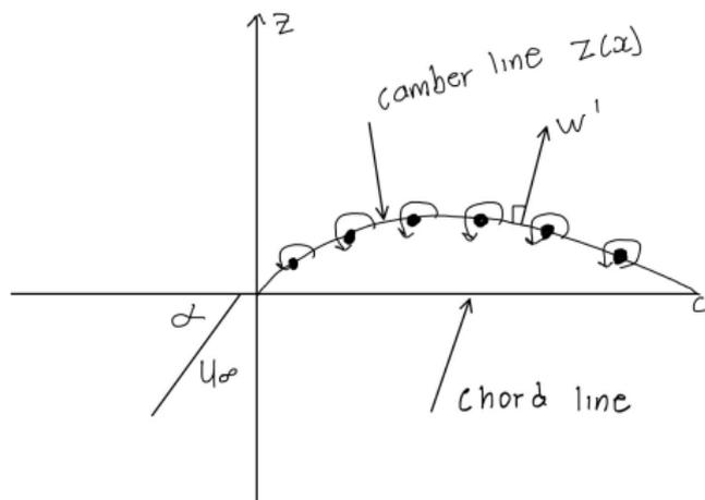
Figure: Vortex sheet on the camber line
