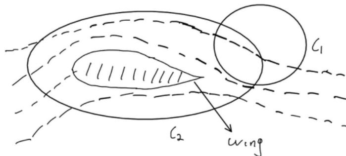
Figure: Two-dimensional irrotational flow
